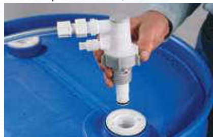
4 Insert coupler into drum insert assembly.
