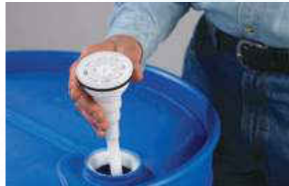
2 Place the drum insert assembly in drum.
