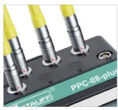
PPC-08-plus with 4 sensor inputs
