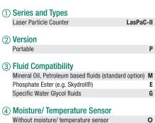
Please note: The moisture/ temperature sensor is not suitable for Phosphate Ester (e.g. Skydrol®) and Water Glycol fluids.
