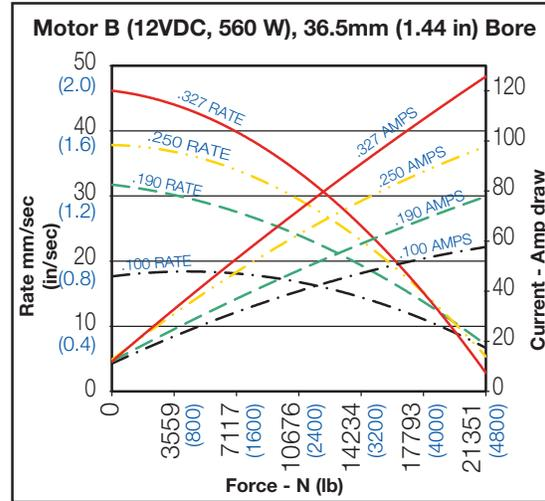
Current draw for Motor C (24VDC, 245 W) and Motor D (24VDC, 560 W) will be approximately 1/2 of Amp draw shown above.
