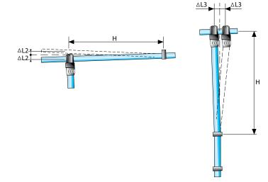
The length variation  $\Delta L$ , calculated for the Transair<sup>®</sup> line, must always be equal to or less than  $\Delta L2$  and  $\Delta L3$ . If this is not the case, then an expansion loop, using Transair<sup>®</sup> flexible hose, must be added.
