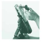
Open the retaining pin at the front of the machine by pressing the jaw to release button\*.
