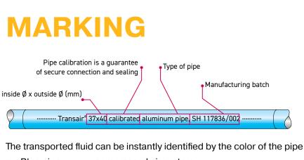
ex: Blue pipe → compressed air system ex: Gray pipe → vacuum system ex: Green pipe → inert gas system
