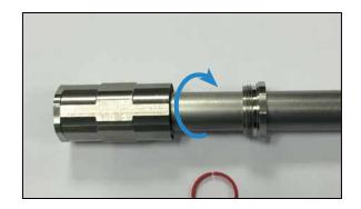
**Disassembly:** 1. Manually unscrew the nut and slide the nut along the pipe.
