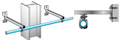
U-channel assemblies are used to offset systems and to bypass obstacles.
