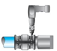
6. Using a drill, fully tighten the clamshell bolts in a cross pattern
