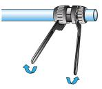
Complete the assembly by tightening the connector onehalf (1/2) turn with the Transair spanner wrenches
