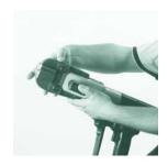
3. Lock into position by closing the retaining pin.
