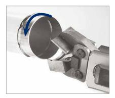
3. Re-open the jaw to remove the pipe. Position the end of the jaw next to the lug mark: this will help to prevent overlapping the lugs.
