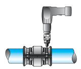
Using a drill, fully tighten the clamshell bolts in a cross pattern Torque Specs: 7.38 lb·ft to 29.5 lb·ft
