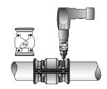
Using a drill, fully tighten the clamshell bolts in a cross pattern Torque Specs: 7.38 lb·ft to 29.5 lb·ft
