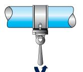
3. Position the plug of the bracket in the hole and tighten the bolts using a crescent wrench
