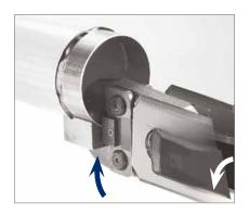
2. Release the jaw then press the trigger and lug the pipe until a "snap" is heard.
