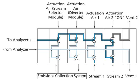
2. The Stream 2 and CEMS Module are in the "on" position. The sample is flowing through CEMS Module to the analyzer.
