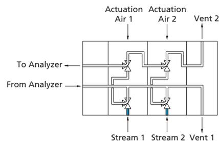
2. When Stream 1 is in the "on" position, the sample flows from Stream 1, through the analyzer, and is routed to Vent 1. Other streams are in the "off" position.
