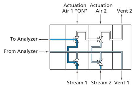
3. When Stream 2 is in the "on" position, the sample flows from Stream 2, through the analyzer and is routed to Vent 1. Other streams are in the "off" position.
