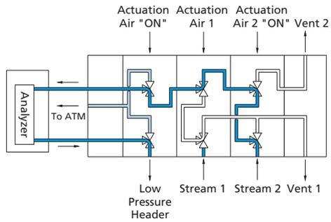
3. Stream 2 is in the "on" position and the ARV Module is in the "off" position, equilibrating the sample loop pressure to atmospheric vent pressure.
