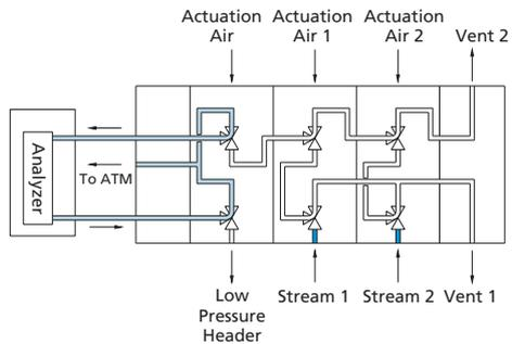
2. Stream 2 and the ARV Module are in the "on" position, purging the sample loop to the low pressure header to ensure representative sampling.
