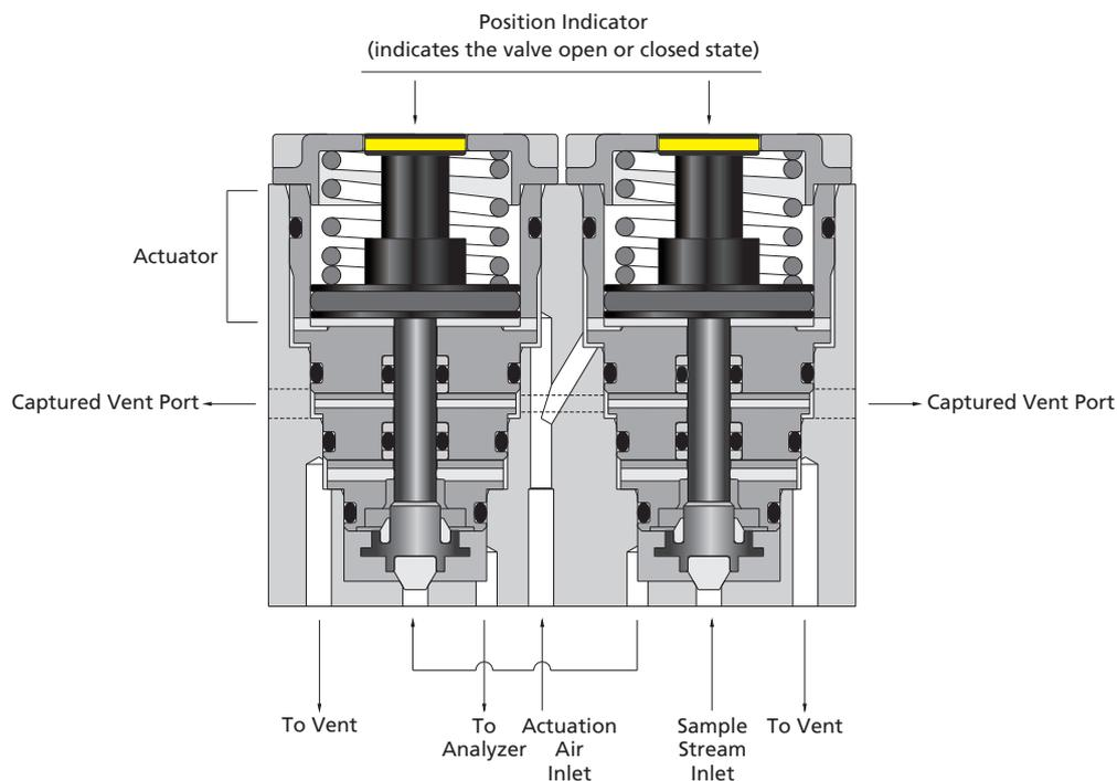
Example shown is a two stream switching system with the flow diagram as follows:
