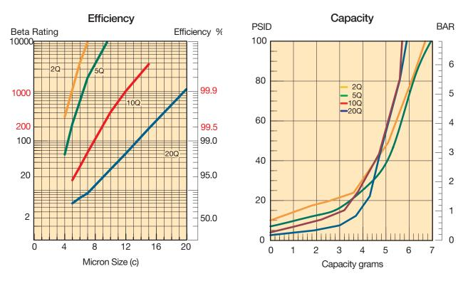
Results typical from Multi-pass tests run per test standard ISO 16889 @ 10 gpm to 100 psid terminal - 10 mg/L BUGL Refer to Appendix on pages 264-265 for relationship to test standard ISO 4572.
