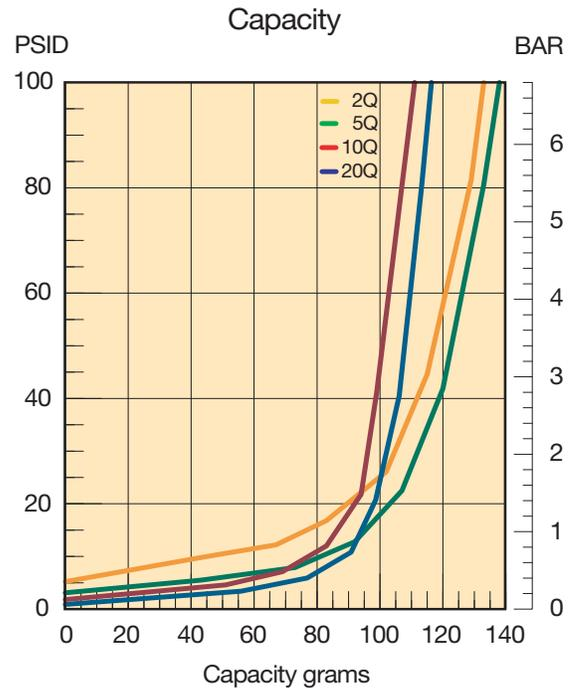
Results typical from Multi-pass tests run per test standard ISO 16889 @ 70 gpm to 100 psid terminal - 10 mg/L BUGL. Refer to Appendix on pages 264-265 for relationship to test standard ISO 4572.
