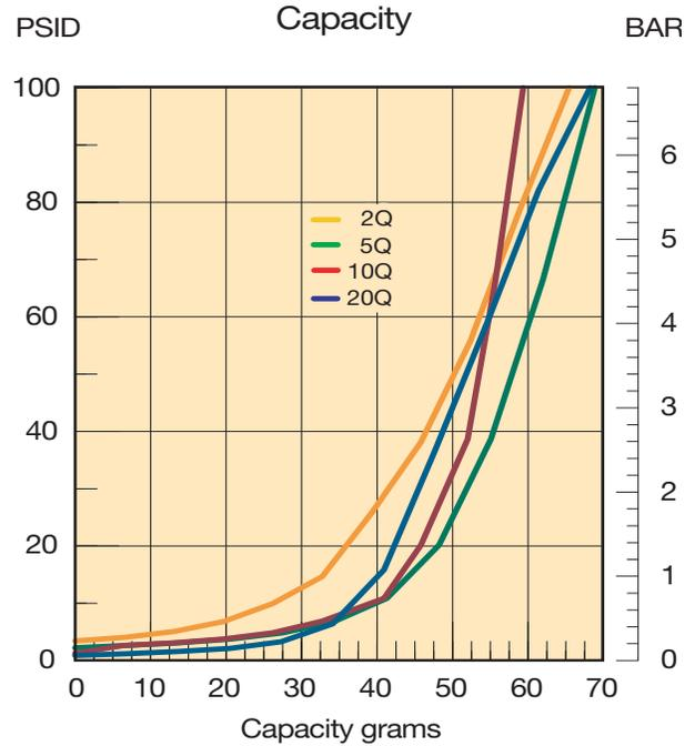
Results typical from Multi-pass tests run per test standard ISO 16889 @ 30 gpm to 100 psid terminal - 10 mg/L BUGL
