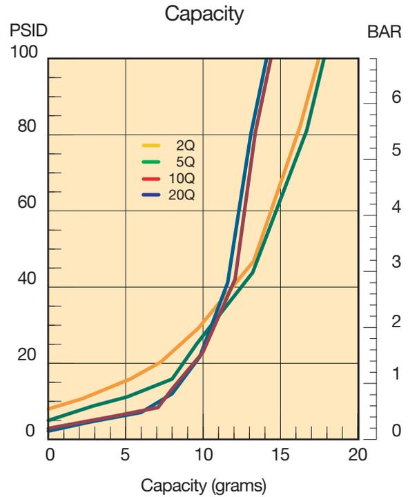
Results typical from Multi-pass tests run per test standard ISO 16889 @ 15 gpm to 100 psid terminal - 10 mg/L BUGL
