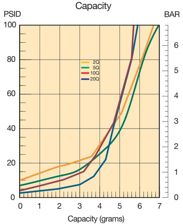
Results typical from Multi-pass tests run per test standard ISO 16889 @ 10 gpm to 100 psid terminal - 10 mg/L BUGL
