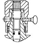
Finger screw Option (Code "F") provides this thumbscrew in place of set screw.
