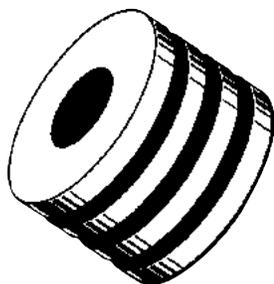
The *one-piece, wide surface*, nodular iron piston reduces bearing loads. The piston is piloted to ensure concentricity. Loctite is used to permanently lock the piston to the rod.
