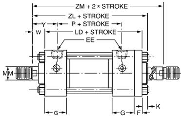
To obtain dimensioning information on a double rod cylinder, first select the desired mounting style and refer to the corresponding single rod cylinder model shown on the preceding pages. After you have determined all necessary dimensions from that drawing, turn back to this page and supplement those dimensions with additional ones from this drawing and the table at right. These added dimensions provide the additional information needed to completely dimension a double rod cylinder model.
