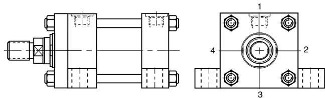
Ports at position 2 or 4 in 25mm to 100mm bore sizes of mounting style C are offset toward position 1 and are not available in the head of 25mm and 32mm bores with number 2 rods. 25mm and 32mm bore heads will not be elongated 5mm toward position 2 or 4 when a port is specified at either of those two locations (the 5mm elongation at position 1 will remain). Contact the factory for the offset dimension.
