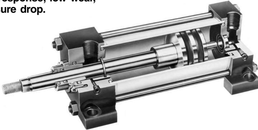
Parker engineers have developed a new concept in air cylinder cushions...the "check seal". The new Parker check seal cushion combines the sealing capabilities of a lipseal for efficient capture of air for effective cushioning with check valve action for quick stroke reversal.
