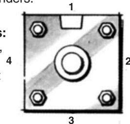
In such special assemblies the cushion needle and check valves are also repositioned because their relation with the port position does not change.
