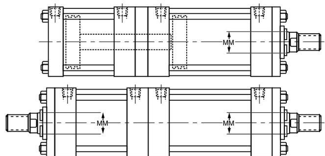
Reduced operating pressure is required for this construction. Contact factory.
