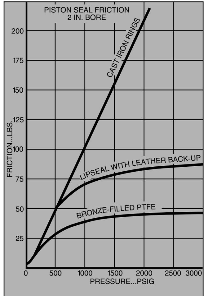
**Virtually zero leakage.** The HI LOAD piston assembly means virtually zero leakage with hydraulic and/or water base fluids because of the continuous bronze-filled PTFE rings with a homogenous inner ring of Nitrile rubber to apply seal preloading. The Nitrile expanders provide enough initial radial force to eliminate low pressure leakage. At higher pressure (above 2,000 psi) the seals are pressurized underneath, and are therefore dynamically self-sealing just as cast iron rings are.
