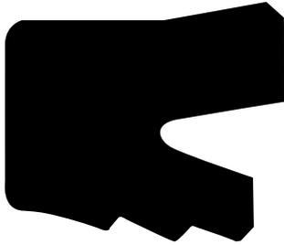
The only fluid adhering to the rod at this point is that very thin layer which is usually “scraped” off the rod on the return stroke by the rugged rod wiper. The solution to this is relatively simple. Don’t let it get out.
