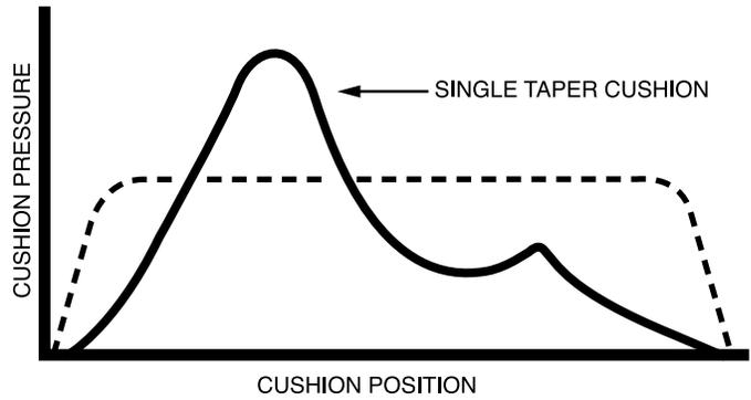
approximate the constant deceleration curve. Pressure peaks are lower than those of both the straight and tapered cushions, resulting in significantly lower hydraulic shock.
