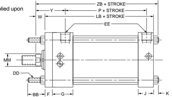
Style TB (NFFA MX3). Head Tie Rods Extended, illustrated: Style TC (NFFA MX2), Cap Tie Rods Extended; and Style TD (NFFA MX1). Both Ends Tie Rods Extended are also available. All "T" styles can be dimensioned from Style TB drawing at right.
