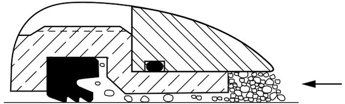
The block vee and hat packing are both low friction type seals and depend upon fine line contact with the rod to effect the seal at a minimum friction value. By scientific optical methods, investigation has indicated this "theory" is short lived as pressure increases. As the pressure increases, the critical edge lifts from the rod, or you might say the line of contact moves away from the pressure.
