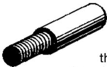
The high strength rod end stud has rolled threads providing threads reducing the possibility of fatigue failure. *Interchangeability*, easy conversion and/or repair of rod ends allow low cost modification or on-the-job repair. Anaerobic adhesive is used to permanently lock the stud to the piston rod.
