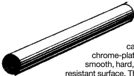
For example, the piston rod is case-hardened and chrome-plated to guarantee a smooth, hard, dent and scratch resistant surface. This increases seal and bearing life, reduces maintenance costs and assures dependable *long-life service*.
