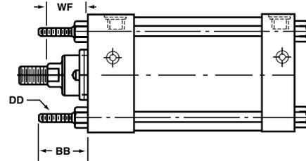
Style TB, Tie Rods Extended, is illustrated at right. Style TC, Cap Tie Rods Extended, and Style TD, Both Ends Tie Rods Extended, can be dimensioned from Style TB drawing.
