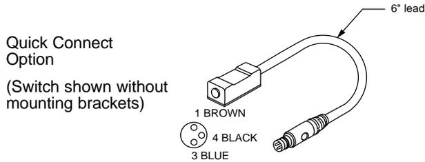
**Switches with 6" Lead and Quick Connect Male End**
