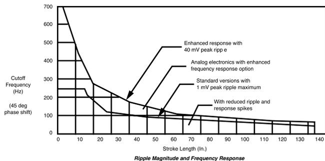
It shows that the AC ripple fundamental frequency is related to stroke length. For shorter strokes, this frequency is usually beyond the response capability of the analog control loop. Notice that the ripple frequency equals the frequency of the interrogation pulse.
