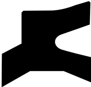
Let’s look at the return stroke now. What happens to the fluid trapped between the Wiperseal and TS-2000 rod seal? (Note the general configuration of the TS-2000 rod seal.)
