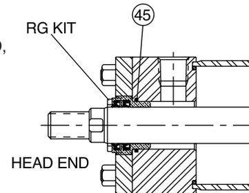
When replacing a gland on a rod which is threaded to the full diameter or so shaped that it could damage the seals, a slight rotary motion of the gland will help prevent damage. In addition, because full-diameter threads are usually supplied with the crest of the threads slightly truncated, a piece of shim stock or other thin, tough material can be wrapped around the threads to help protect the gland seals when they are being passed over the threads.
