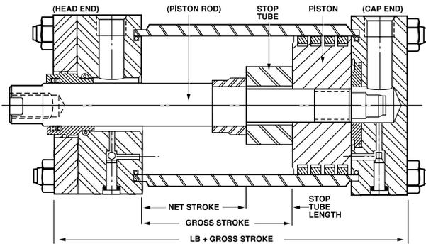
When specifying cylinders with long stroke and stop tube, be sure to call out the net stroke and the length of the stop tube. Machine design can be continued without delay by laying in a cylinder equivalent in length to the NET STROKE PLUS STOP TUBE LENGTH, which is referred to as GROSS STROKE. Refer to piston rod/stroke selection chart to determine stop tube length.
