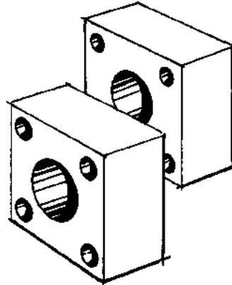
Square Steel heads and caps provide concentricity for mating parts. Both the steel head and cap are bored and grooved to assure concentricity to a common centerline for the cylinder body.
