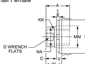
A high strength rod end stud is supplied on thread style 4 through 2" diameter rods and on thread style 8 through 1 3/8" diameter rods. Larger sizes or special rod ends are cut threads. Style 4 rod ends are recommended where the workpiece is secured against the rod shoulder. When the workpiece is not shouldered, style 4 rod ends are
