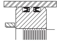
Standard on 50mm bore sizes and larger, Parker's B style piston is a single seal design which incorporates two wear strips. This design provides smooth operation, long bearing life, and high load carrying capacity.
