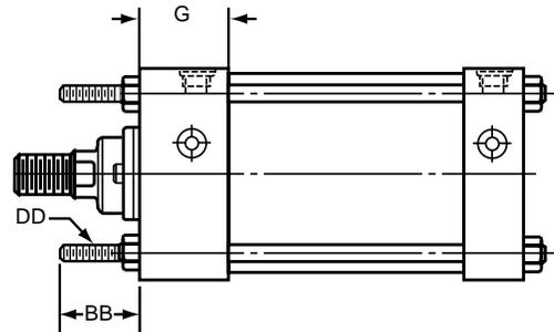
Style TB, Tie Rods Extended, is illustrated at right. Style TC, Cap Tie Rods Extended, and Style TD, Both Ends Tie Rods Extended, can be dimensioned from Style TB drawing.
