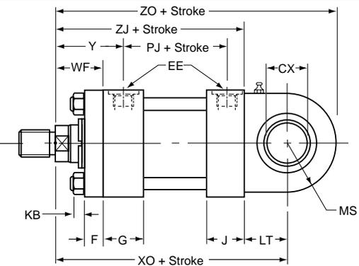
\*Head depth increased by 5mm to accommodate port on 25mm and 32mm bore cylinders – see page 111
