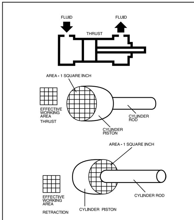
**Pistons** vary in design and materials used. Most are made of cast iron or steel. Several methods of attaching the piston to the rod are used. Cushions, are an available option on most cylinders and most often, can be added with no change in envelope dimensions.
