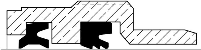
The Parker "Jewel" gland cartridge is a combination of elements designed exclusively for sealing fluids when used in conjunction with reciprocating shafts.
