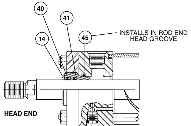
When replacing a gland on a rod which is threaded to the full diameter or so shaped that it could damage the seals, a slight rotary motion of the gland will help prevent damage. In addition, because full-diameter threads are usually supplied with the crest of the threads slightly truncated, a piece of shim stock or other thin, tough material can be wrapped around the threads to help protect the gland seals when they are being passed over the threads.
