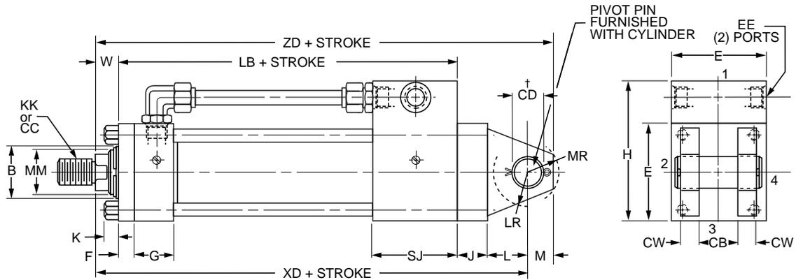
**Cap Spherical Bearing**
