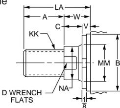
A high strength rod end stud is supplied on thread style 4 through 2" diameter rods and on thread style 8 through 1 3/8" diameter rods. Larger sizes or special rod ends are cut threads. Style 4 rod ends are recommended where the workpiece is secured against the rod shoulder. When the workpiece is not shouldered, style 4 rod ends are
