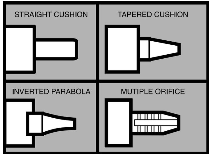
addition, the clearance annulus must be concentric so the fluid flow characteristics remain consistent from one stroke to the next. Parker cylinders use floating bushings and floating cushion sleeves to assure concentricity of the flow annuli. Some designs, however, do not provide the floating feature, thereby increasing the chances of eccentricity of mating cushion parts. When cushion parts do not mate concentrically on each cycle, undercushioning or erratic cushioning results.
