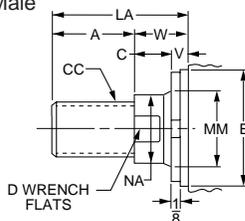
recommended through 2" piston rod diameters and style 8 rod ends are recommended on larger diameters. Use style 9 for applications where female rod end threads are required. If rod end is not specified, style 4 will be supplied.
