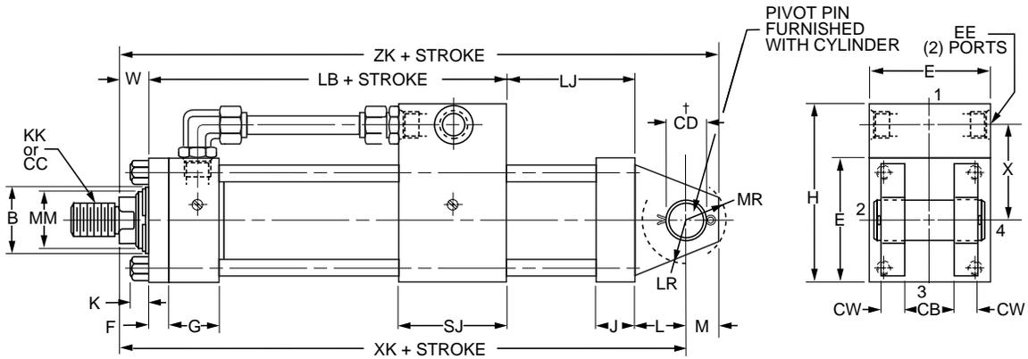
**Cap Spherical Bearing**
