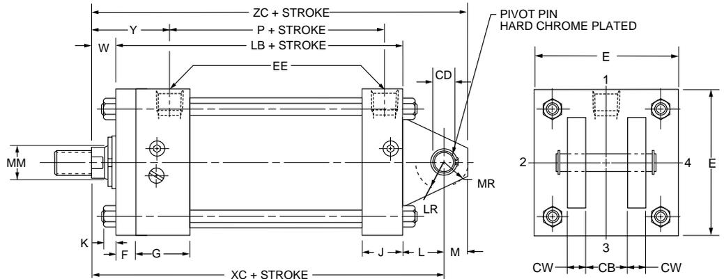
The 1", 4", 5" and 6" bore sizes have tie rod nuts at both ends as shown. Tie rods thread into cap on all other bore sizes.
