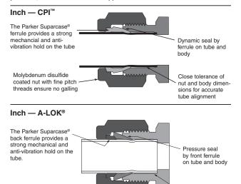
Parker Instrumentation Tube Fittings are supplied complete and ready to use. The ferrule(s) swage onto the tube as it moves down the body seat creating a pressure/vacuum-tight seal on both tube and body by the interface pressure and surface finish of mating components. The Parker Suparcase® ferrule (back-ferrule only on A-LOK®) creates a strong mechanical hold on the tube.
