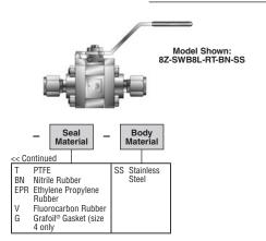
Example: 8A\*-SWB8L-RT-BN-SS describes a SWB8L Two-Way Ball Valve with 1/2" A-LOK® end connections for ports 1 and 2, reinforced PTFE seats, Nitrile rubber body seals, and stainless steel construction.
