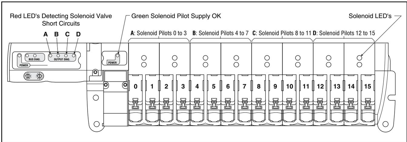
Inside the bus module, solenoid valve control is protected against short-circuits with the following visual indication provided:
