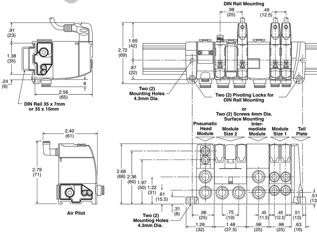
**Special Case:** 4/3 all ports blocked function within island version, add the dimensions of the dual P.O. check valve module plugged into the island.
