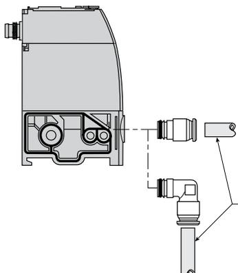
**Fitting Assembly:** Pneumatic Connectors are retained by a clip in each module. Assembly is achieved by pushing the fitting into the module and sliding the clip down over the groove in the fitting. Pull fitting to check that it is secure.
