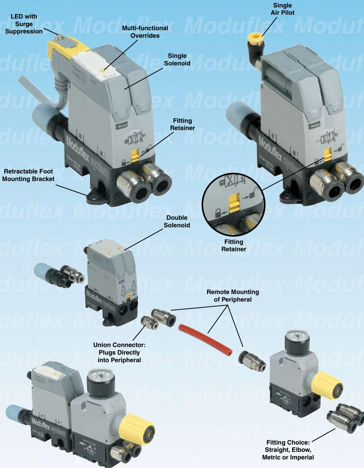
Peripheral modules may either be plugged in the valve output ports or mounted in-line separate from the valve.
