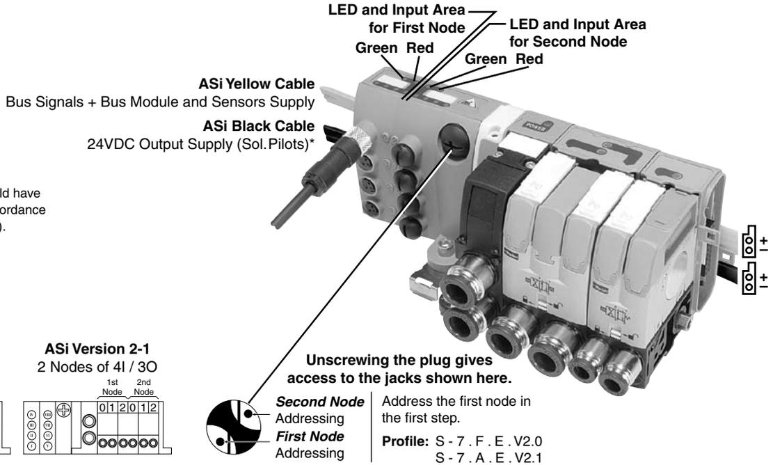
\* The external supply should have protective isolation in accordance with IEC 364-4-41 (PELV).
