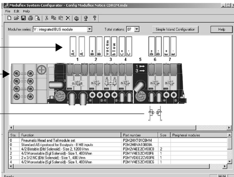
With the Moduflex Valve Island Configurator CD-ROM, you may configure the Moduflex V or T series valve islands that a given application requires.
