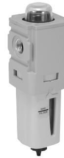
**Note:** To optimize the life of coalescing element, it is advisable to install a P31F pre-filter with a 5 micron element upstream of the coalescing filter.
