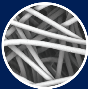
Standard polyester felt magnified 300 times.
