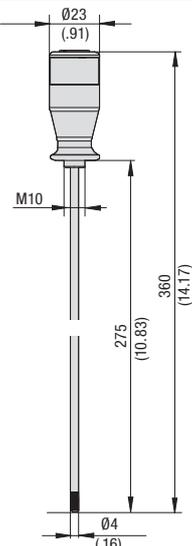
Screw-in Temperature Sensor (T) Process Connection M10x1 Process Connection G1/4 Rod-type Temperature Sensor (TSH)
