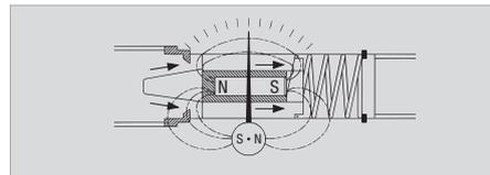
The flow indicators SDM and SDMKR have a sharp-edged orifice and a tapered metering piston, which moves in proportion to changes of flow against a spring. In no flow condition the piston closes the opening and the pointer indicates zero.
