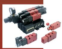
**The C7** is a four-way manifold mounted and body ported, two/three position (5/2 5/3) valve, with  $\frac{1}{4}$ " NPT ports standard and ISO G thread optional. The manifold mounted valves are designed to be mounted on a stacking style manifold and can be manual, pilot or electrically operated with a variety coil options, as well as the Plug-In feature. An optional Pre-Wired sub D connector can support up to 12 valves on a manifold.
