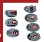
**Overrides** Four types of overrides are available: Standard, Suffix Detail -G, -M and -CML. The standard is a push twist to lock, requires no call out. -G is a guarded momentary contact, -M is an unguarded momentary contact and -CML is a raised grip, push twist to lock.
