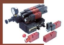
**The C5** is a four-way manifold mounted and body ported, two/three position (5/2 5/3) valves, with 1/8" NPT ports standard and ISO G thread optional. The manifold mounted valves are designed to be mounted on a stacking style manifold and can be manual, pilot or electrically operated with a variety coil options, as well as the Plug-In feature. An optional Pre-Wired sub D connector can support up to 12 valves on a manifold.
