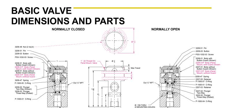
\* Maximum panel thickness is 7/16" except for valves without button guard. For theses, maximum panel thickness is 1/4".
