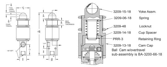
Can be operated by a cam or machine member. Has 3/16" overtravel after full actuation. This valve can be panel mounted. Pressure angle should not exceed 15° from vertical center line. Cam follower is hardened 430F stainless steel.
