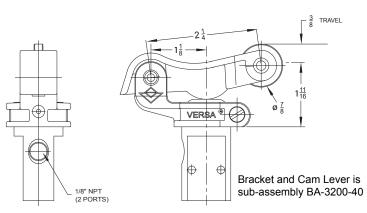
Actuated by cam movement in either direction. Cam follower is hardened.
