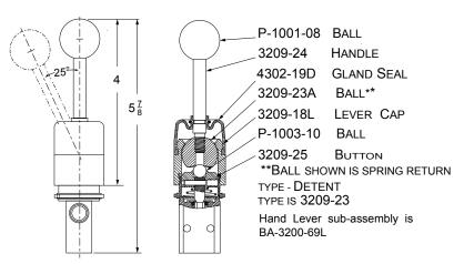
Light force, offsetting the handle  $25^{\circ}$  from vertical, is sufficient to operate
