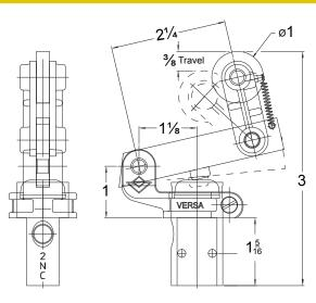
Bracket and Trip-Cam Lever is sub-assembly BA-3200-40-35.
